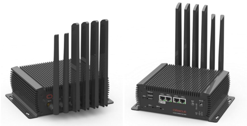
Image 2: Oracle Cloud Connector 5G + Wi-Fi Antennas
